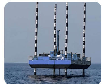
GEOTECHNICAL INVESTIGATION USING MODULAR PONTOON AND SPECIALIZED MARINE EQUIPMENT
